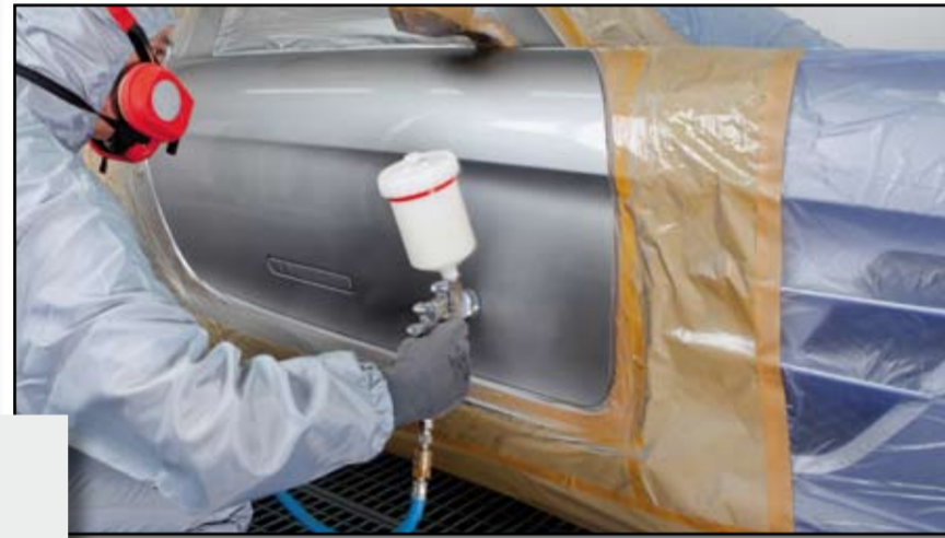
Applying the 2K Special Matt ready to use clearcoat mixture in two carefully controlled overlapping coats with inter-coat flash-off 5 – 10 minutes.
