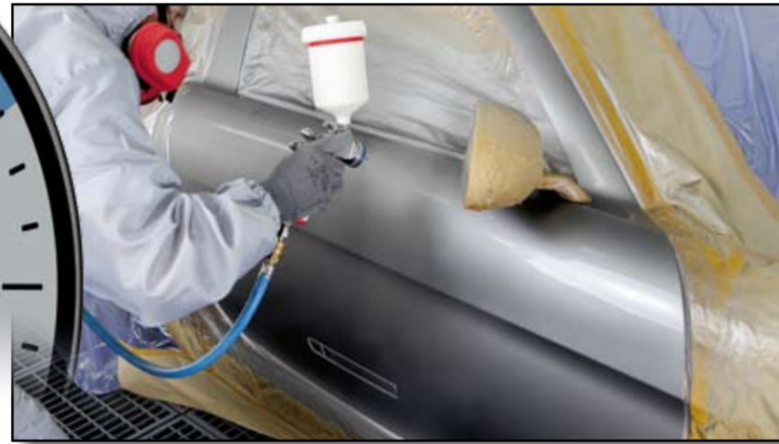
Applying the 2K Special Matt ready to use clearcoat mixture in two carefully controlled overlapping coats with inter-coat flash-off 5 – 10 minutes.
