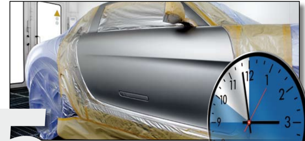
Drying the matt clearcoat 45 – 50 minutes at 60°C object temperature.
